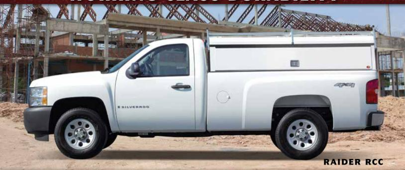
**Raider RCC (Commercial Cap)** Functional and affordable, Raider Commercial Caps (RCC) offer you the best commercial canopy available today. The RCC comes standard with a Super Cage Roof Design with integrated Mounting Rail, Heavy-Duty TIG Welded Frame and Stainless Steel Folding T-Handles. With a full array of options including custom paint, tool boxes, full size doors and double side doors, the RCC can be tailored for your specific needs.
